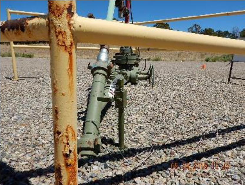
Photo 3: Unused steel 1" riser at 1A.
