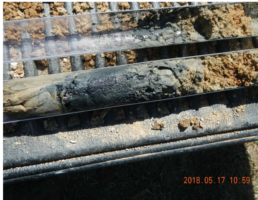
Photo #4 – Soil sample included a hydrocarbon smear zone
