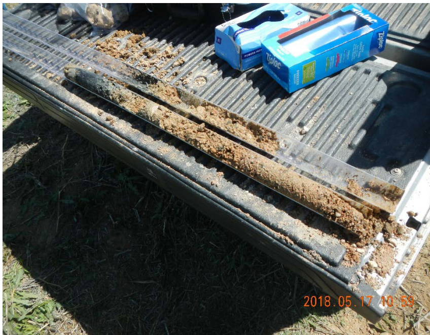
Photo #5 – Soil sample including hydrocarbon smear zone
