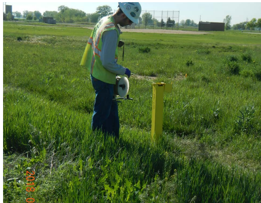
Photo #2 – Gauging monitoring wells prior to using Geoprobe
