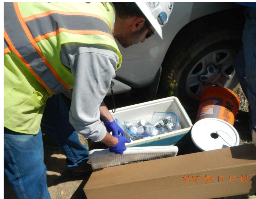
Photo #6 – Soil samples selected for lab analysis being stored in a cooler, on ice.
