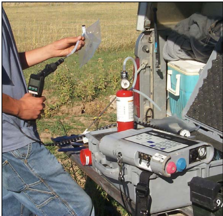
Figure 2. A Foxborough TVA 1000 flame/photo ionization detector (FID/PID) was used to check around plugged and abandoned wells for oil and gas seeps. The instrument was calibrated with ambient air (0 ppm) and 100, 1,000, 10,000 and 50,000-ppm standards. The PID was calibrated with ambient air a 100-ppm isobutylene standard. Instrument checks were repeated several times a day to monitor for drift.
