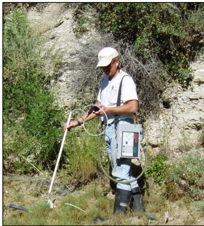
Figure 2. A Foxborough TVA 1000 flame/photo ionization detector (FID/PID) was used to check around plugged and abandoned wells for oil and gas seeps. The instrument was calibrated with ambient air (0 ppm) and 100, 1,000, 10,000 and 50,000-ppm standards. The PID was calibrated with ambient air a 100-ppm isobutylene standard. Instrument checks were repeated several times a day to monitor for drift.
