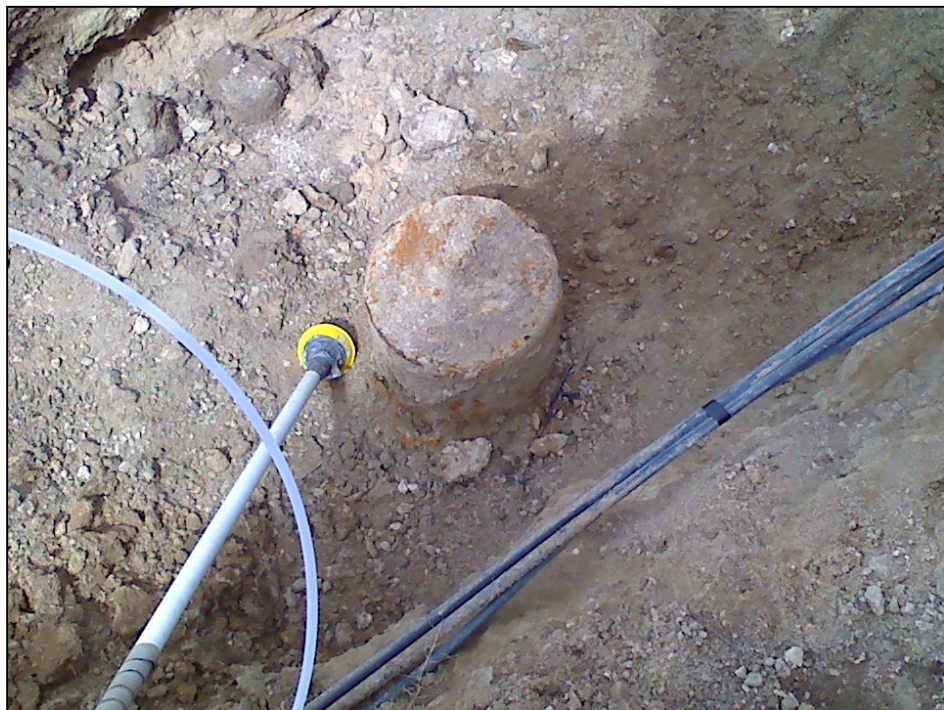
Figure 2. A Foxborough TVA 1000 flame/photo ionization detector (FID/PID) was used to check around plugged and abandoned wells for oil and gas seeps. The instrument was calibrated with ambient air (0 ppm) and 100, 1,000, 10,000 and 50,000-ppm standards. The PID was calibrated with ambient air a 100-ppm isobutylene standard. Instrument checks were repeated several times a day to monitor for drift.
