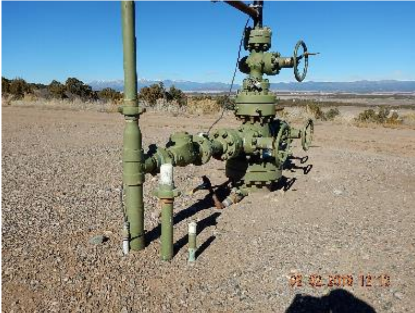
Photo 5: Risers at wellhead previous inspection.
