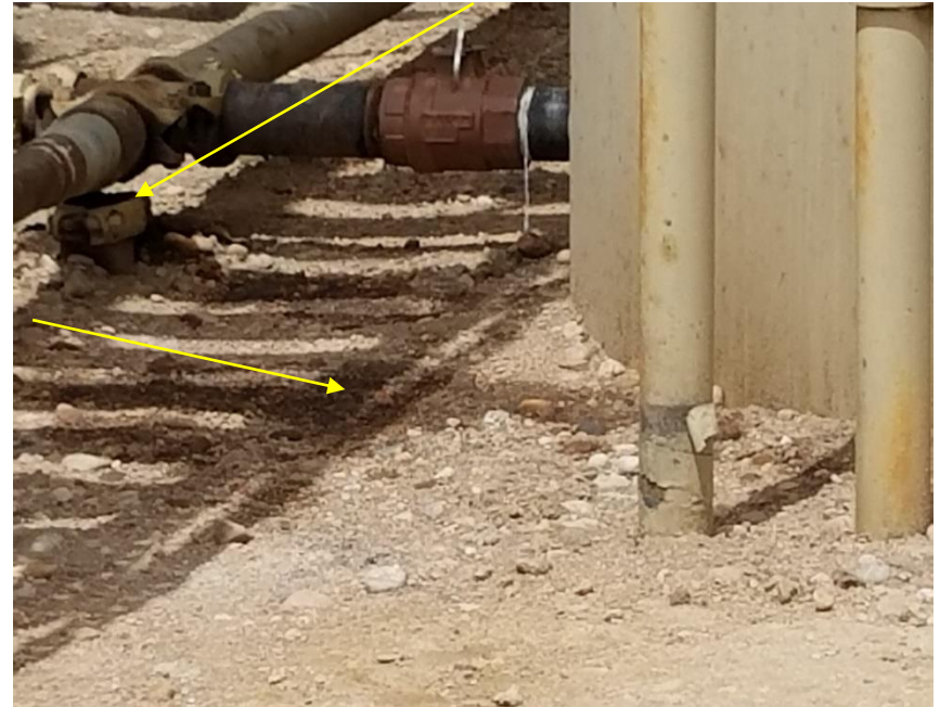
Photo 4. Unmarked riser and stained soil center of crude oil Tanks
