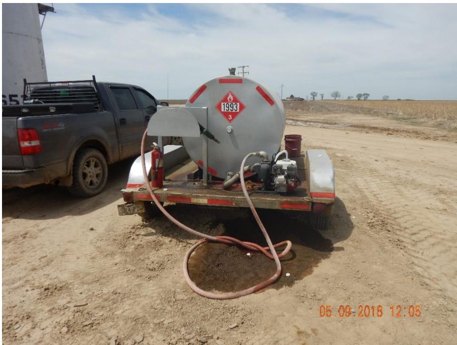
Photo 1: Photo taken from the north end of the location, facing west. Photo shows what looks to be a fuel tank w/ pump containing diesel fluids appears to be leaking onto the pad. Fluids can be found over the trailer as well as ponding beneath.
