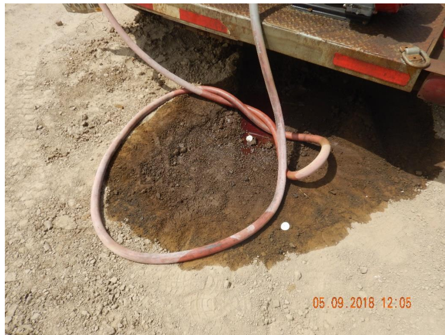
Photo 2: Photo taken from the north end of the location. Photo shows what looks to be a fuel tank w/ pump containing diesel fluids appears to be leaking onto the pad. Fluids can be found over the trailer as well as ponding beneath.
