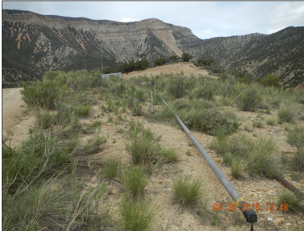
Out of service flow lines.
