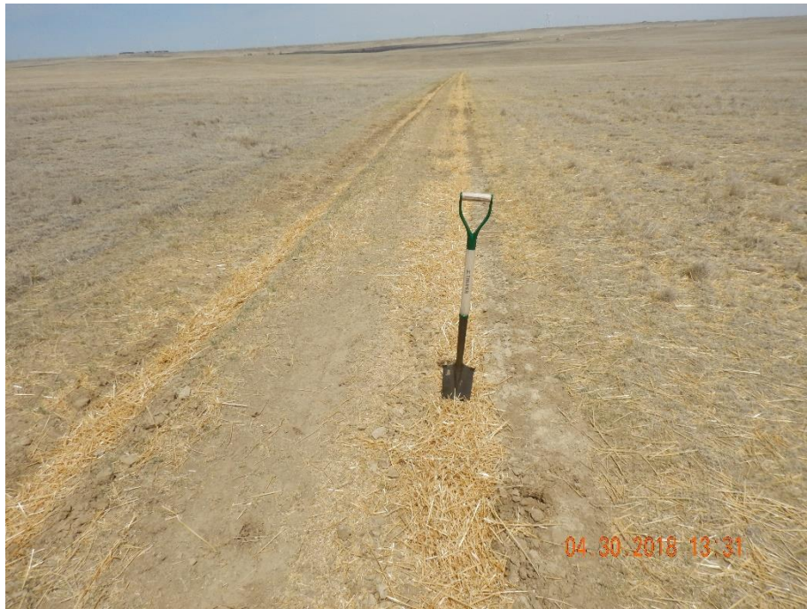
Photo 7: Photo taken from the access road, facing northeast. Photo shows inspector tested the access road for compaction concerns. Photo shows soils within the areas of the ruts, where a ripper did pass through, were easier to penetrate.
