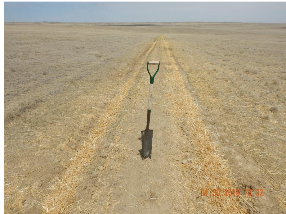
Photo 8: Photo taken from the access road, facing northeast. Photo shows inspector tested the access road for compaction concerns. Photo shows soils OUTSIDE the areas of the ruts, where a ripper DID NOT pass through, were difficult to penetrate; inspector was only able to easily penetrate to top couple inches of soil. Compaction concerns remain evident.
