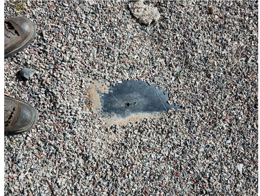
Location photo #4 Holes in tank battery containment
