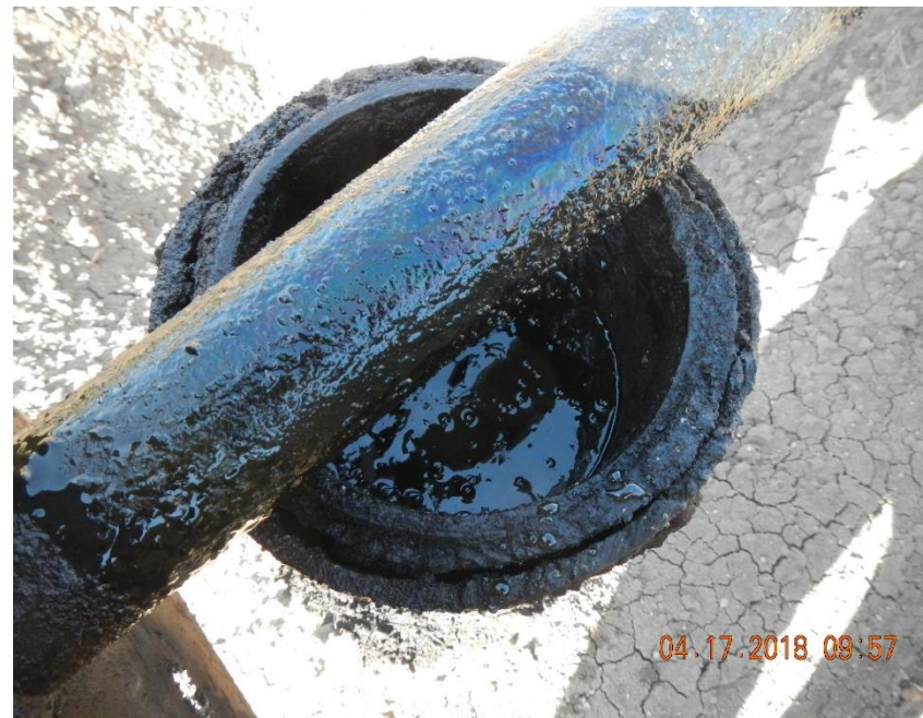
Fluids present in Fitzhugh #7 well bore. PA marker is not welded on.
