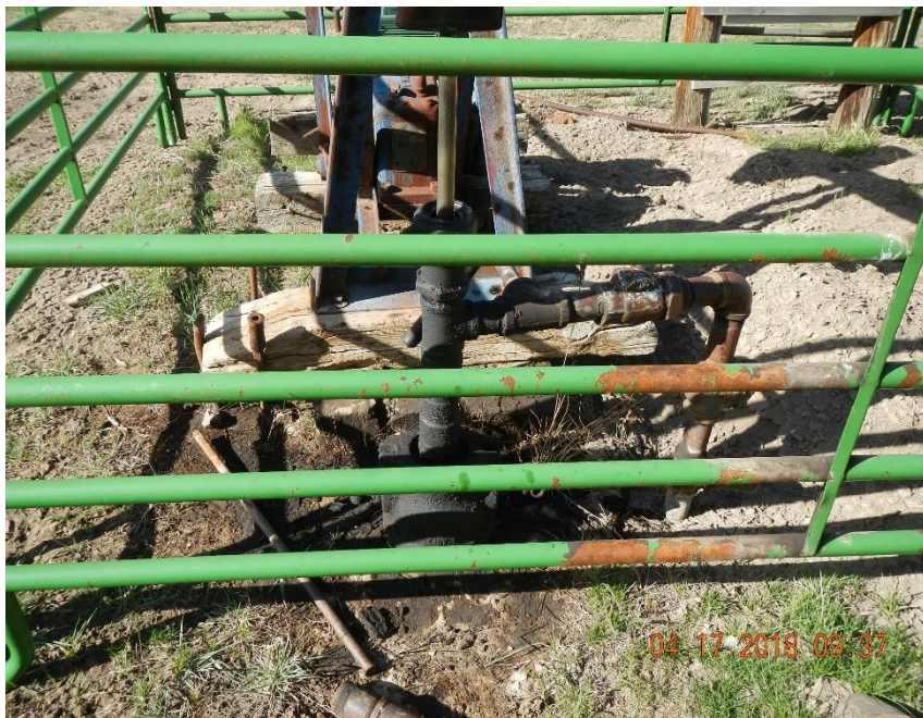
Fitzhugh #6 well head and surrounding soil are stained.
