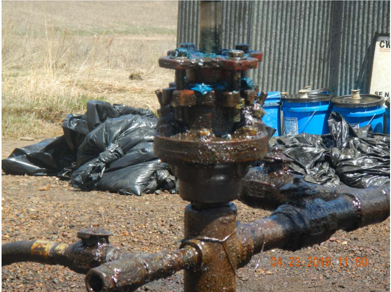
Wellhead, freshly greased packing
