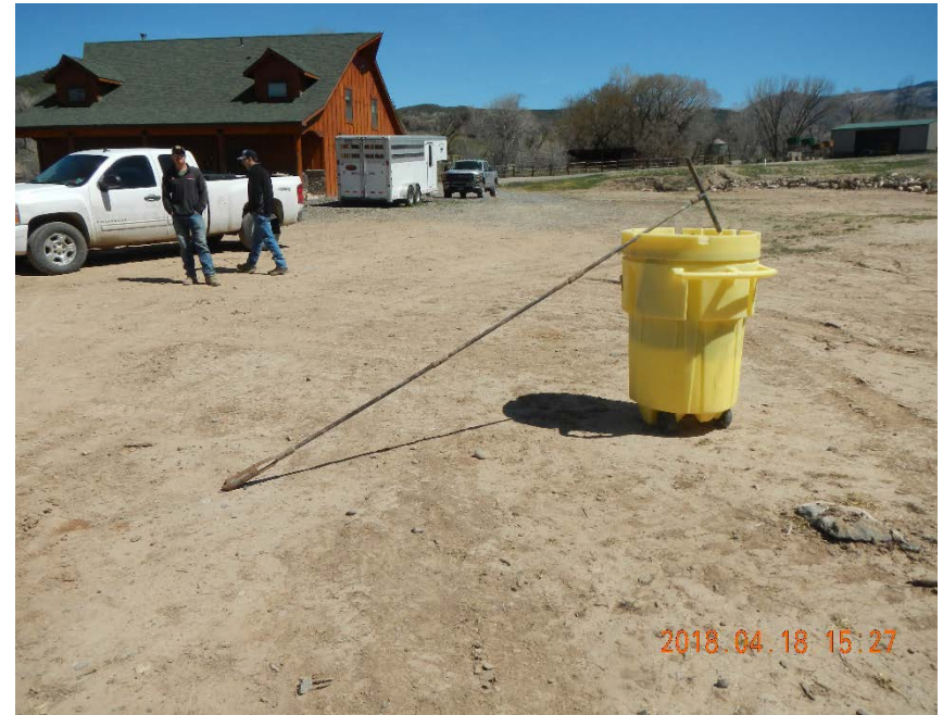
Hand auger used to take samples around the excavation, along the pipeline pathway (on both directions) and downgradient.
