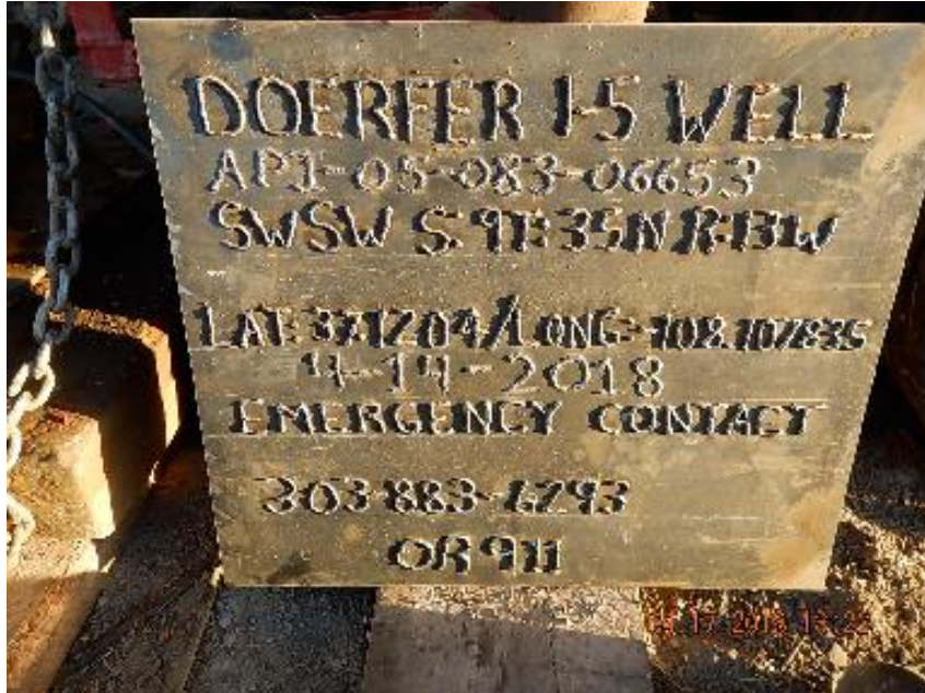
Photo 7: Plug and abandon marker.
