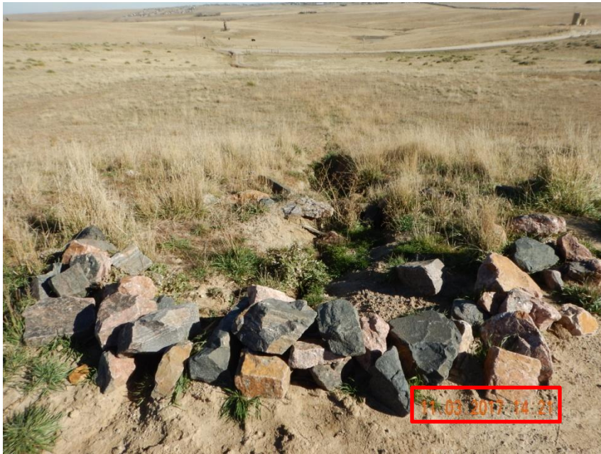
Photo 1. Photo taken from the northeast well pad on November 3, 2017, facing East. Rip-rap has been installed but does not appear to be a sufficient BMP as active gully erosion is evident. Operator needs to repair gully erosion and install sufficient BMPs.
