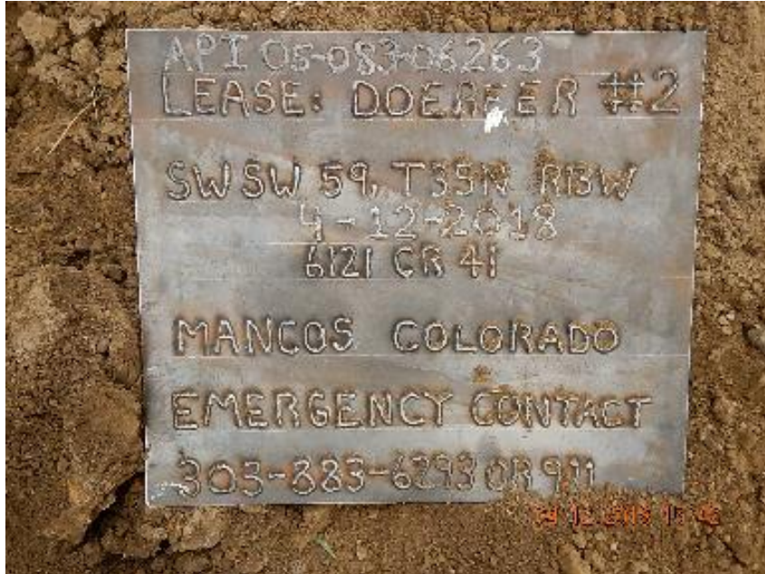
Photo 7: Plug and abandon marker.
