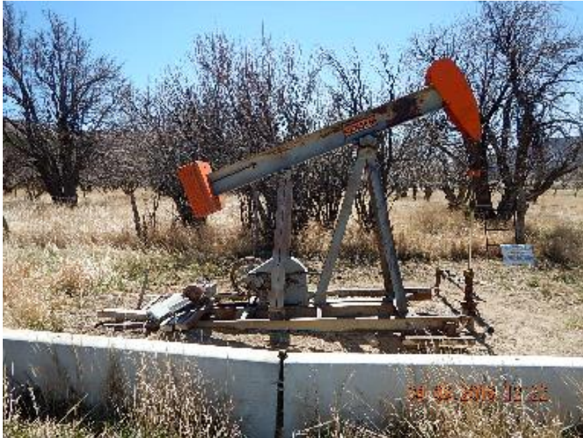
Photo 3: Pump jack and electrical equipment.
