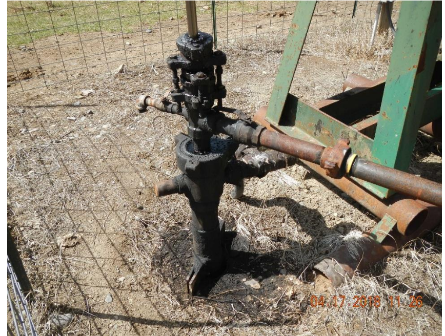
Well head and surrounding soil is stained with oil.
