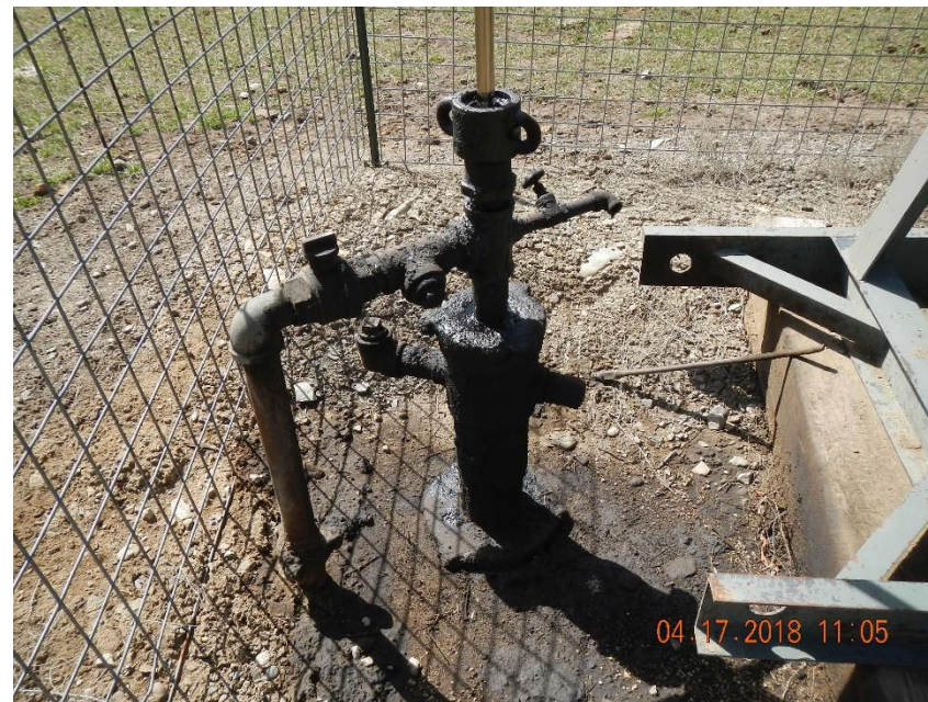
Well head and surrounding soil stained with oil .
