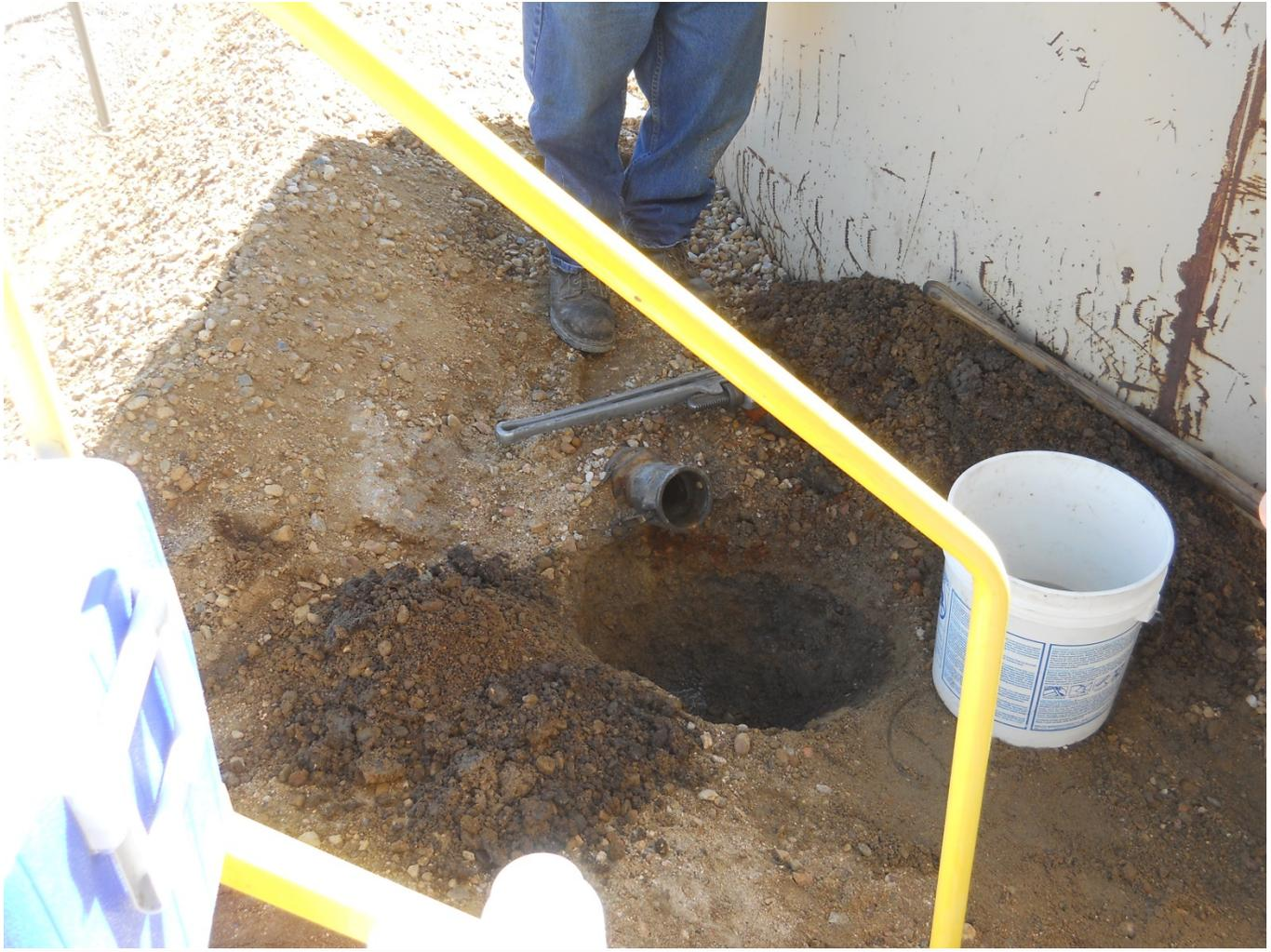
In the photo above the operator excavated a shallow hole to allow the disposable plastic bucket to receive produced water from the tank. Samples were poured into lab provided containers using a funnel as shown previously.
