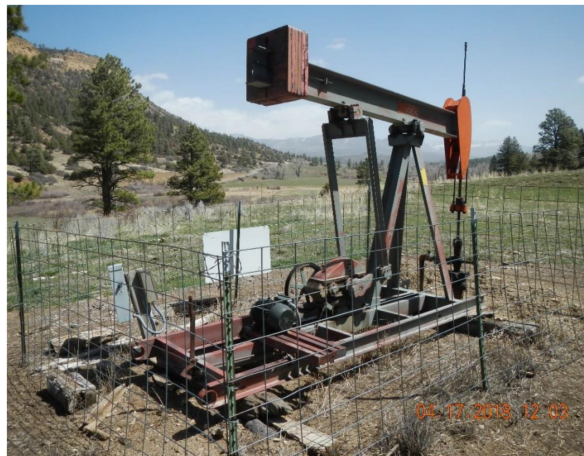
Chavez #2 pump jack and electric prime mover.
