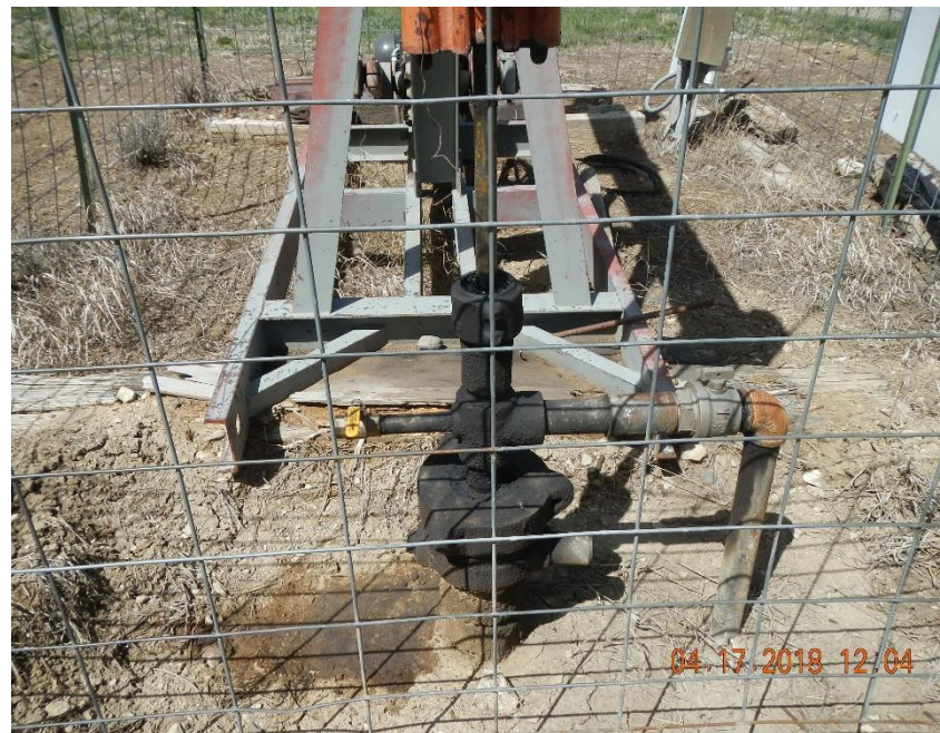
Oil stained well head and soil.
