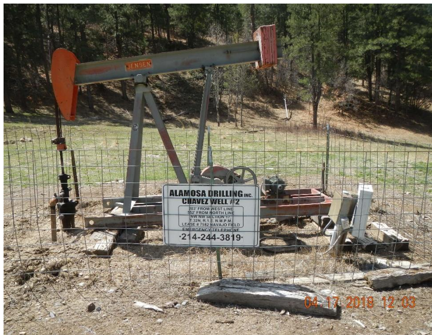
Chavez #2 well head and pump jack.
