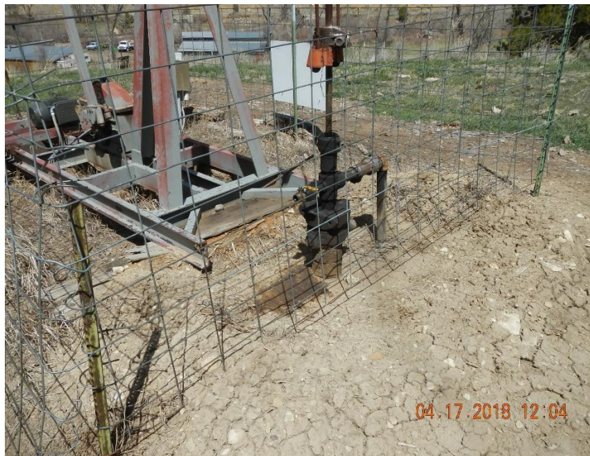
Well head and area below valve are stained.
