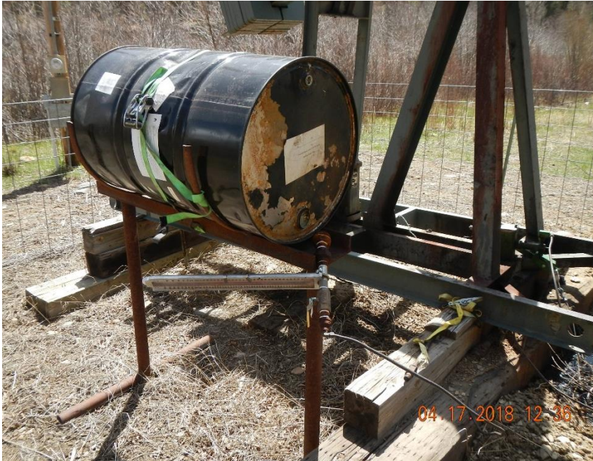
Unused 55 gal. drum chemical injection system.
