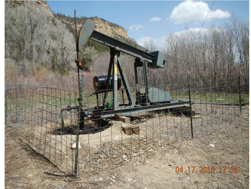
Nielson #3 well head and pump jack.
