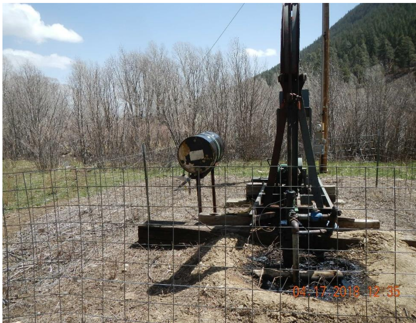
Nielson #3 well head with oil staining.
