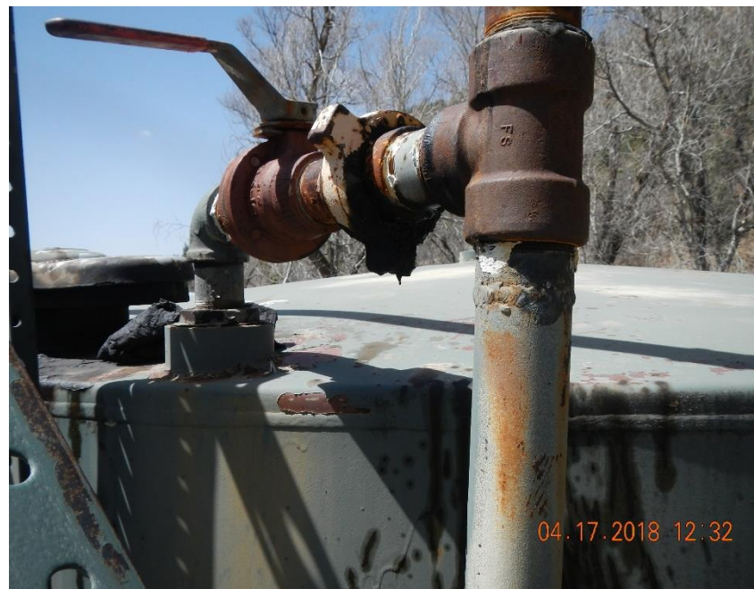
Leaking hammer union on flow line.
