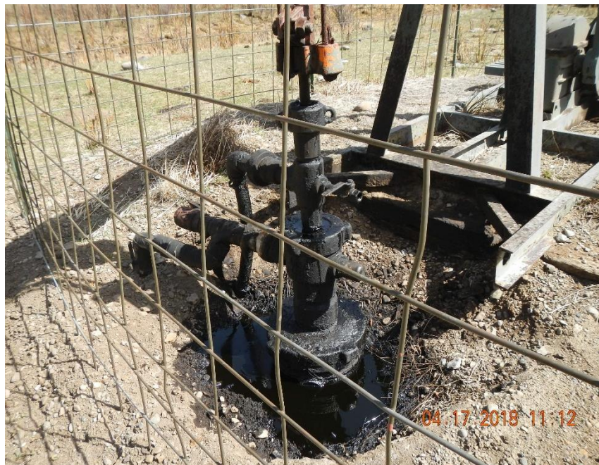
Nielson #5 well head is wet and stained with oil.
