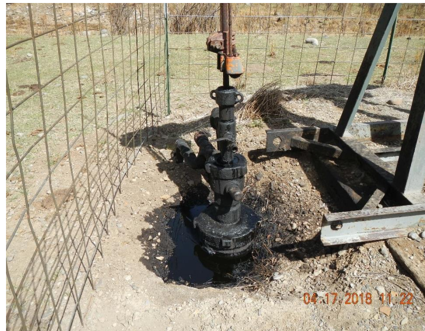
Well head and surrounding soil wet with oil.
