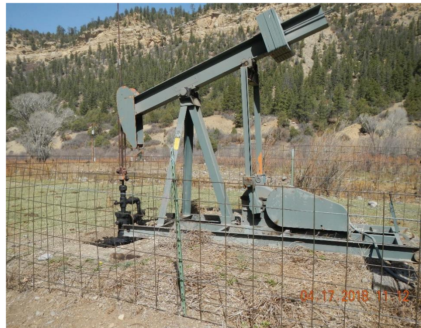
Nielson #5 pump jack and stained well head.
