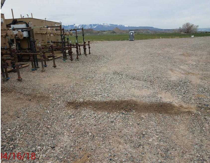
Location photo # 3 Stained soil by separators
