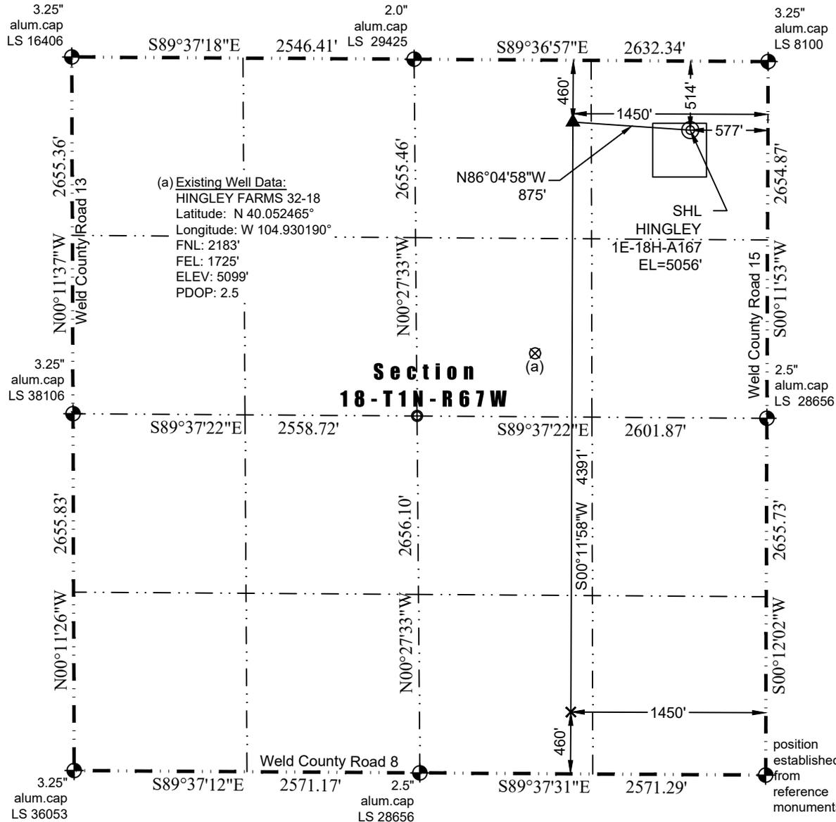
In accordance with a request from Jay Knutson of Crestone Peak Resources, Washburn Land Surveying, LLC has determined the location of the **Hingley 1E-18H-A167** well site to be SHL: 514' FNL and 577' FEL, (TPZ: 460' FNL and 1450' FEL, BHL: 460' FSL and 1450' FEL), as measured at ninety (90) degrees from the section lines of Section 18, Township 1 North, Range 67 West of the 6th Principal Meridian, Weld County Colorado.
