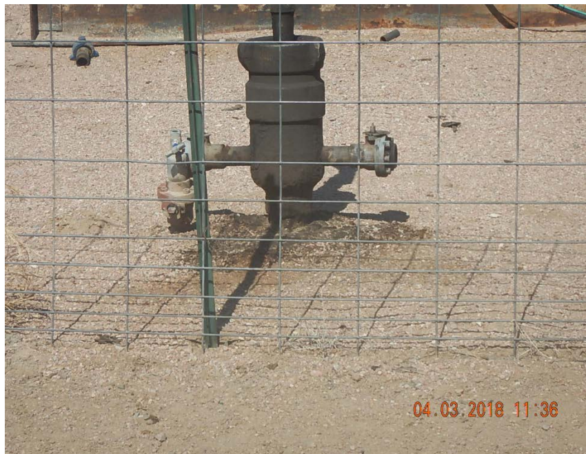
Photo 3: Stained soil at wellhead
