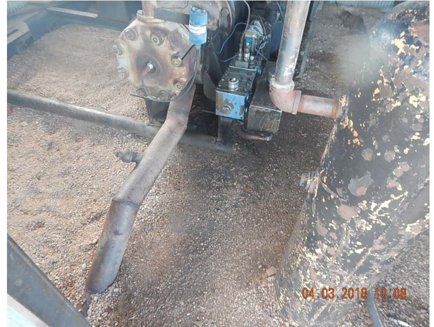
Photo 4: Stained soil at engine
