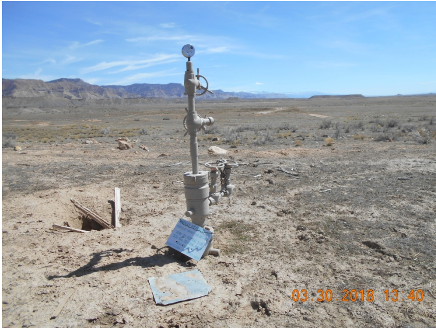
TA wellhead with sign.
