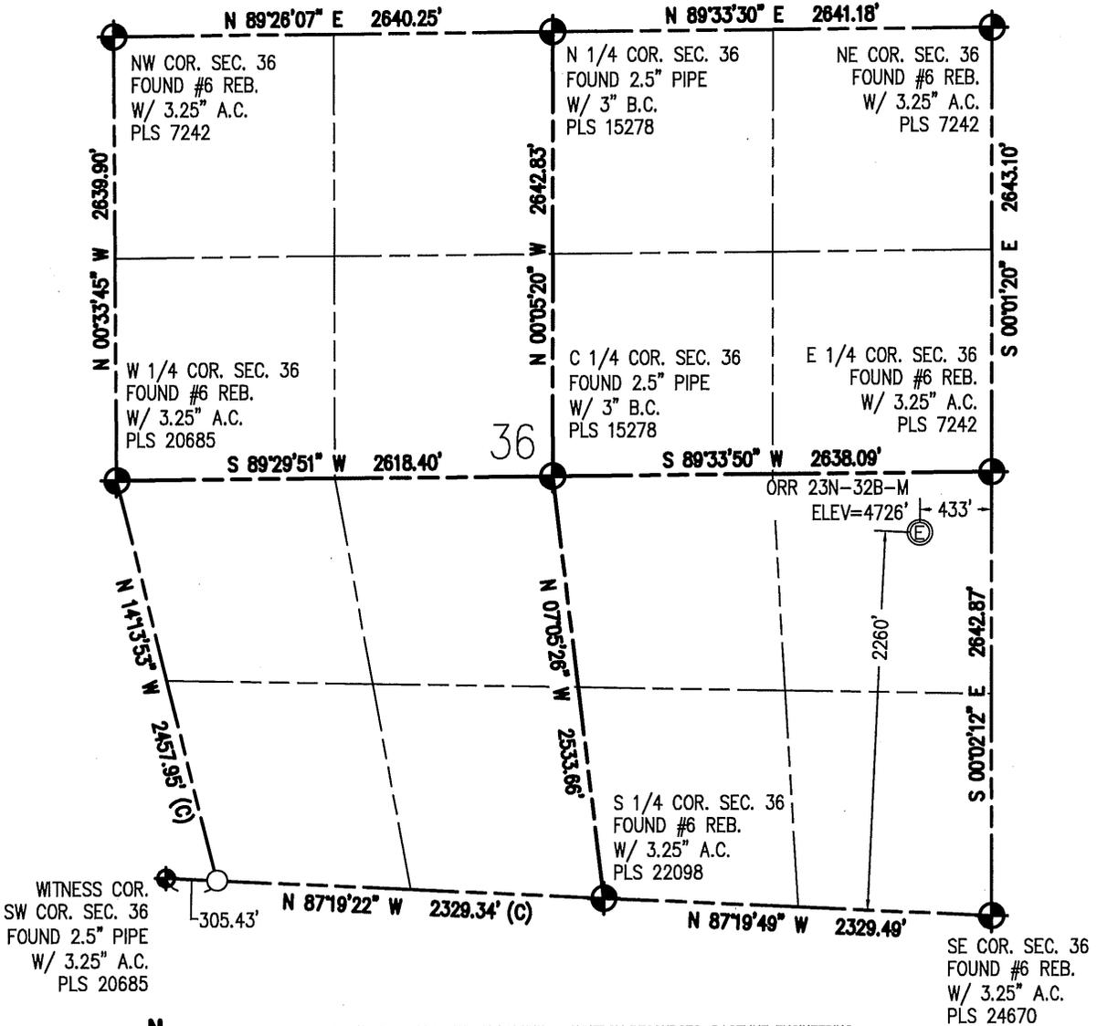
**N** IN ACCORDANCE WITH A REQUEST FROM BRANDON LORENZ - SYNERGY RESOURCES, BASELINE ENGINEERING CORP. HAS DETERMINED THE LOCATION OF THE ORR 23N-32B-M TO BE 2260' FSL AND 433' FEL, AS MEASURED AT NINETY (90) DEGREES FROM THE SECTION LINE OF SECTION 36, TOWNSHIP 6 NORTH, RANGE 67 WEST, 6TH PRINCIPAL MERIDIAN, WELD COUNTY, COLORADO.
