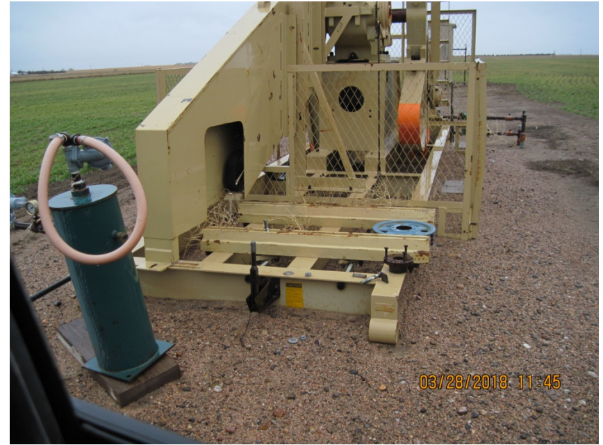
4. Prime mover has been removed
