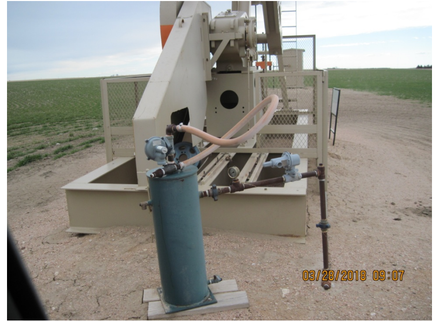
2. Prime mover has been removed
