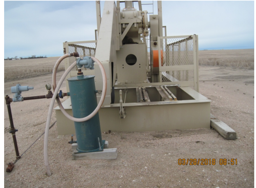
2. Prime mover has been removed
