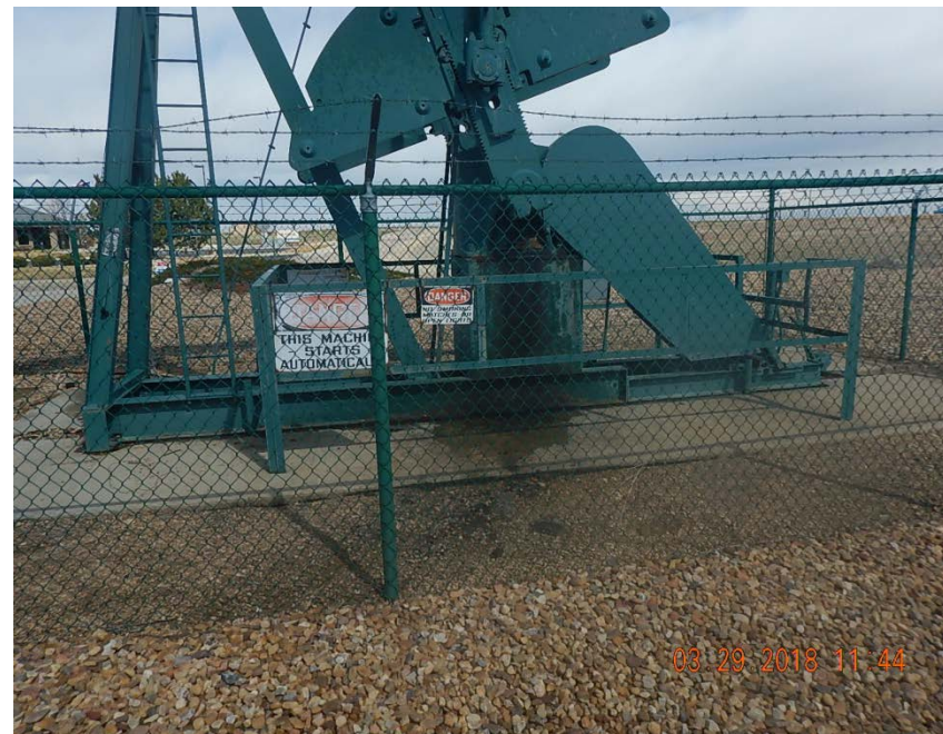
Photo 2: Staining at gearbox
