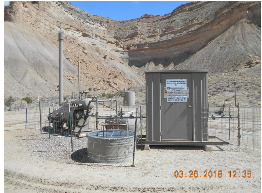
Separator, Meter housing with fencing
