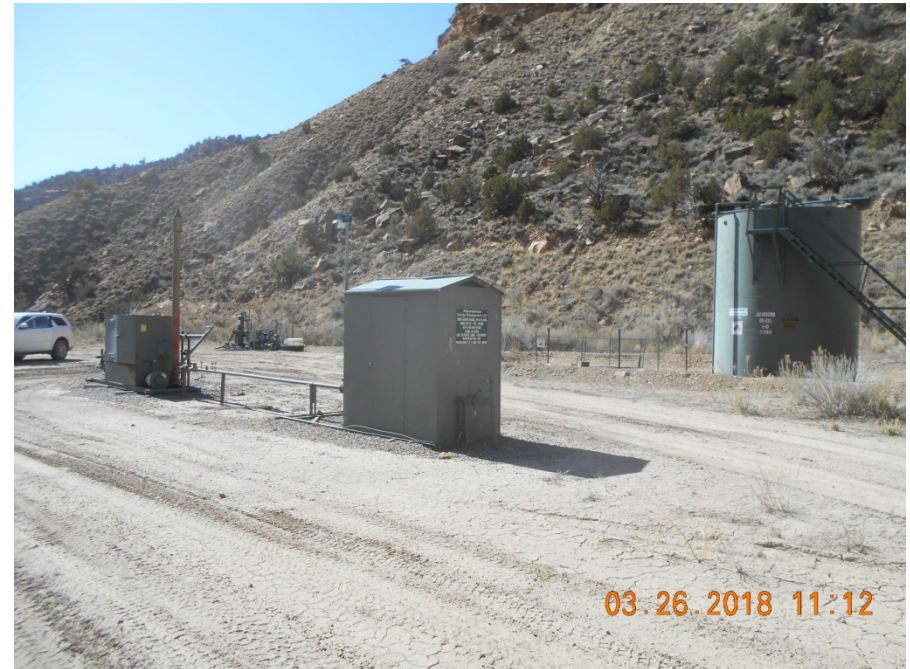
Separator and Meter housing.
