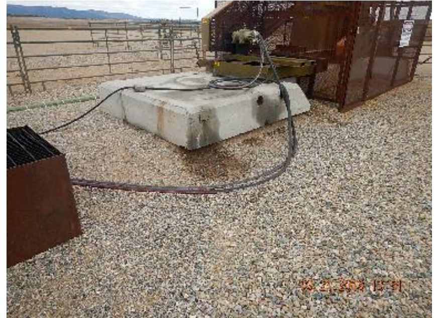
Photo 8: Impacted soil and gravel at rear of concrete base of pump jack.
