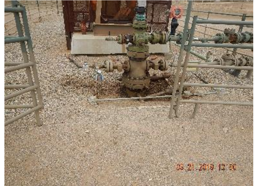
Photo 4: Impacted soil and gravel around base of wellhead.
