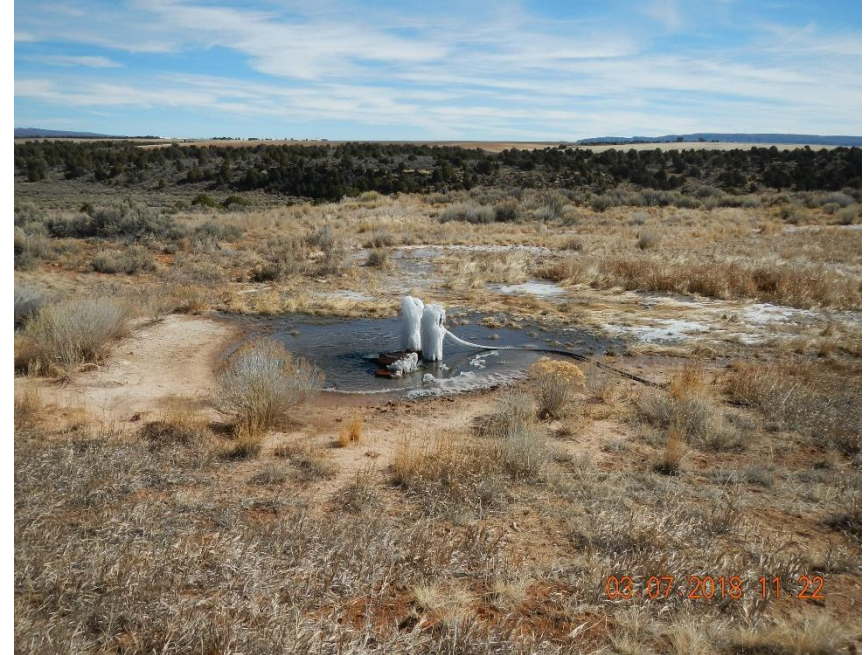
Cathodic protection well releasing gas and water.
