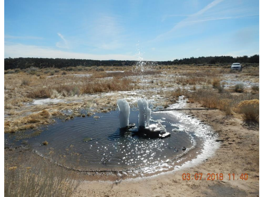
Cathodic protection well intermittently spraying water into the air.
