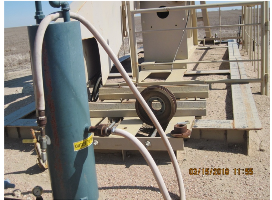
4. Prime mover has been removed.
