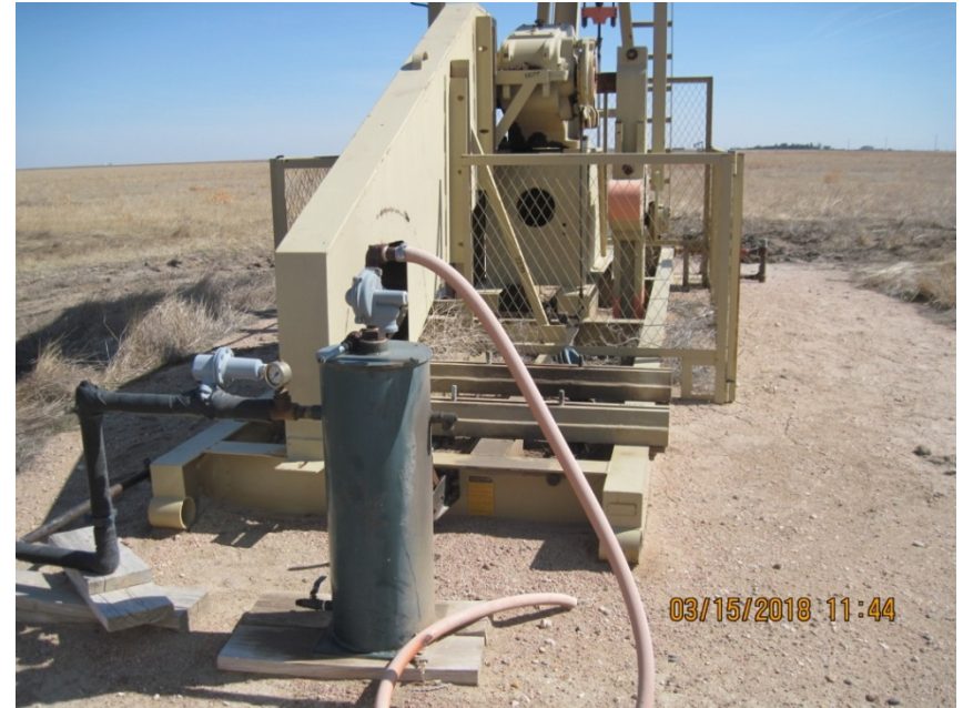
4. Prime mover has been removed.
