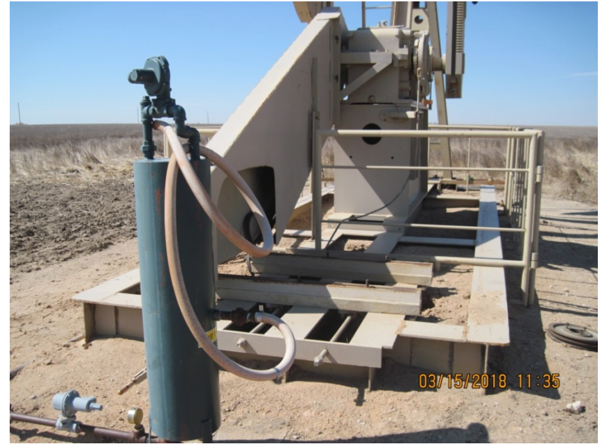
4. Prime mover has been removed.
