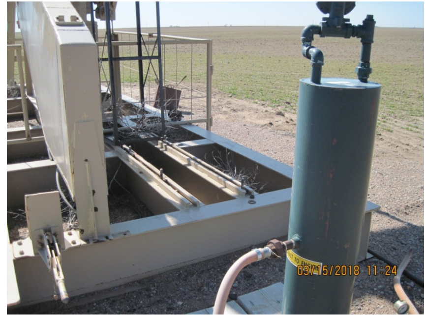
4. Prime mover have been removed.
