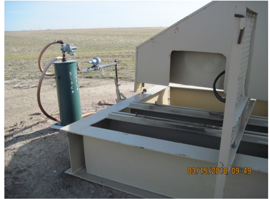
4. Prime mover has been removed
