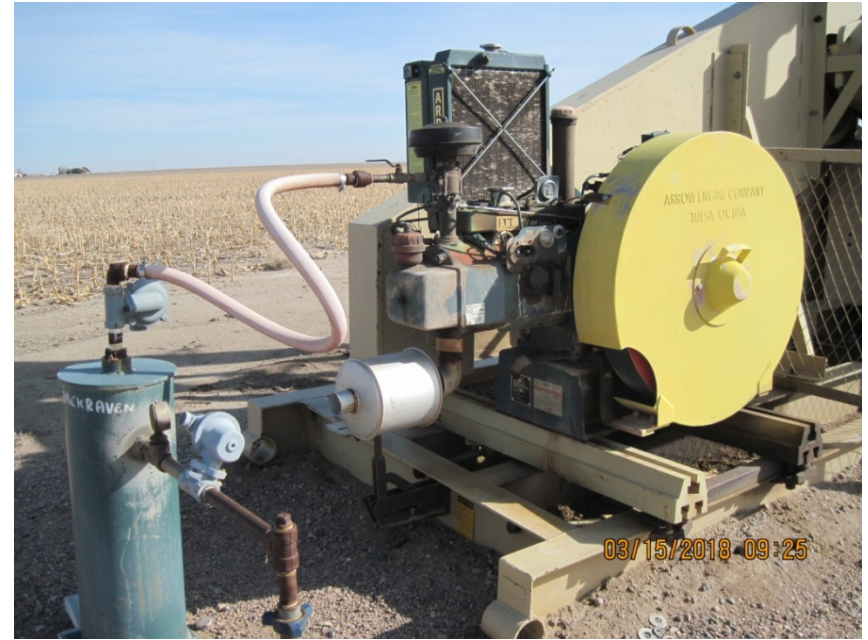
4. Prime mover, C-66 Arrow gas engine
