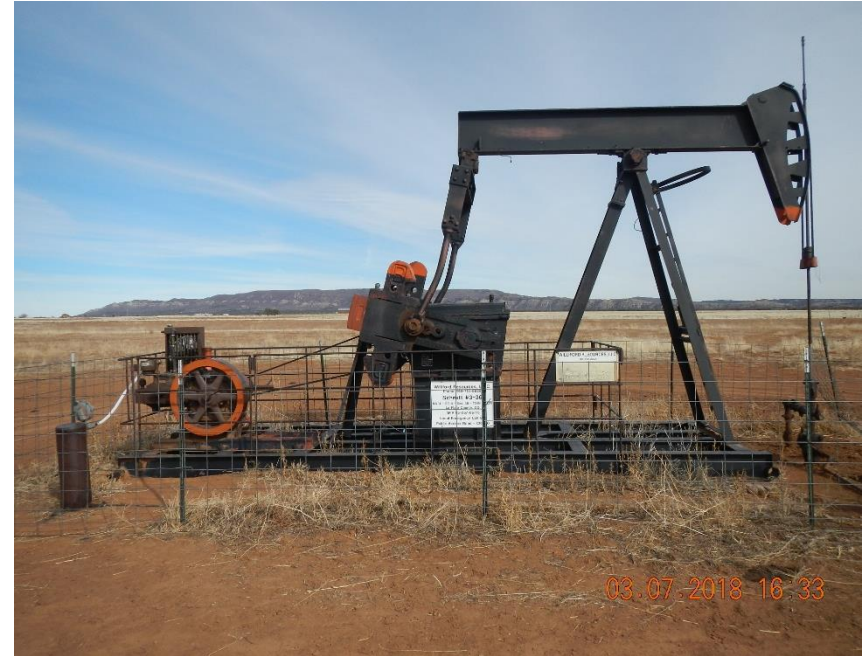
Schmitt #3-36 pump jack and well head.
