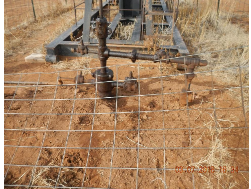
Well head is wet and surrounding area is stained.
