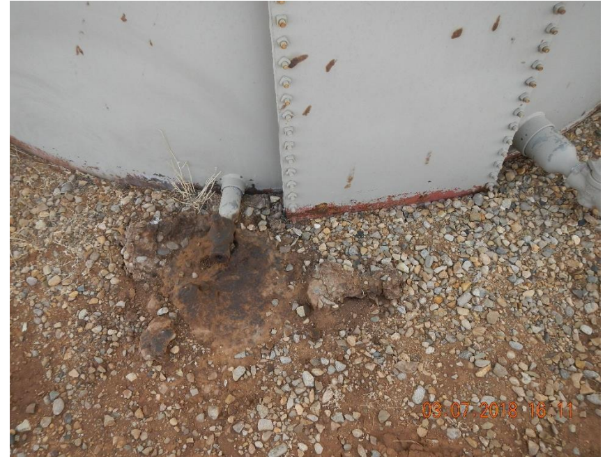
Stained soil below tank valves.
