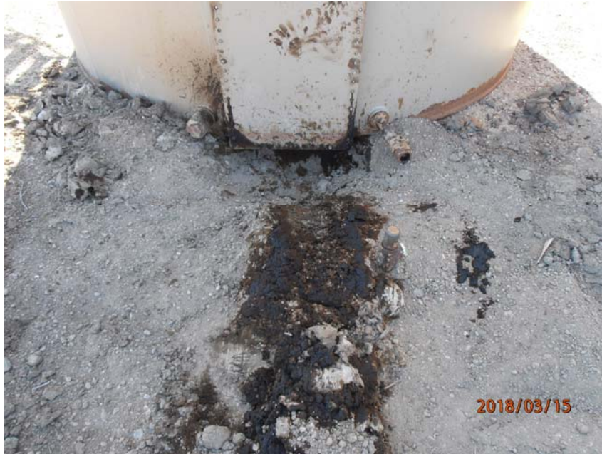
Photo 5 – North side of eastern crude oil AST. Oily material extends beneath tank.
