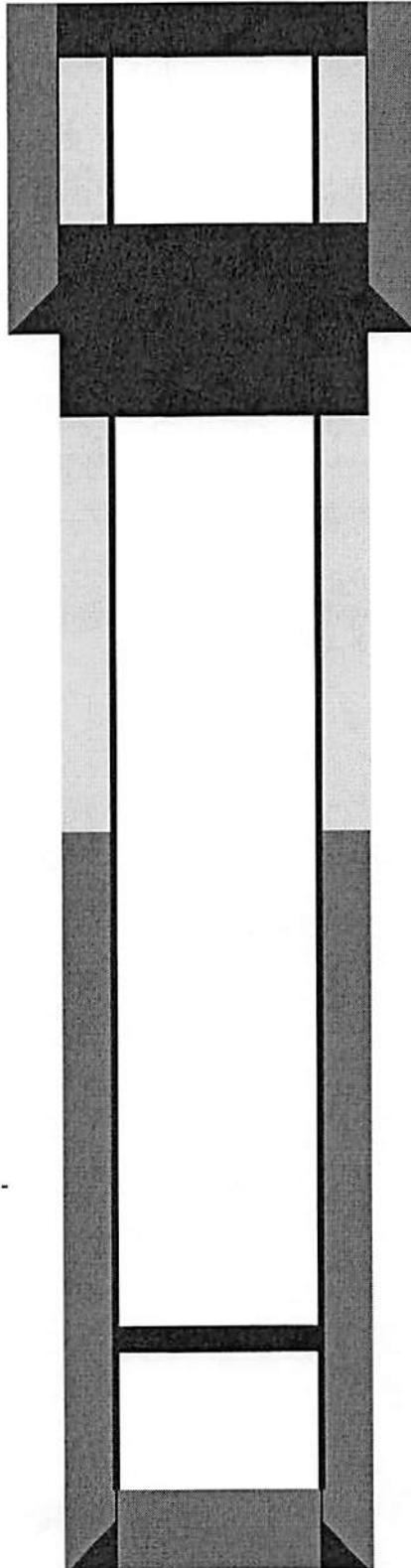
Use 1" tubing to spot 20 sxs of cement in the casing from 50' up.
