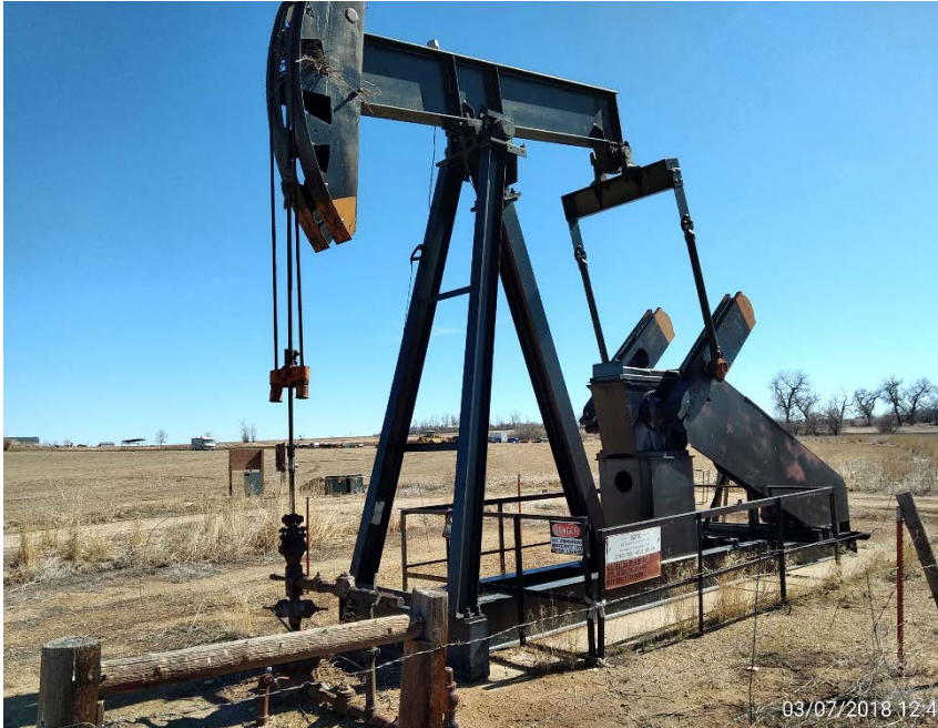
Wellhead, Pumping Unit, & Prime Mover
