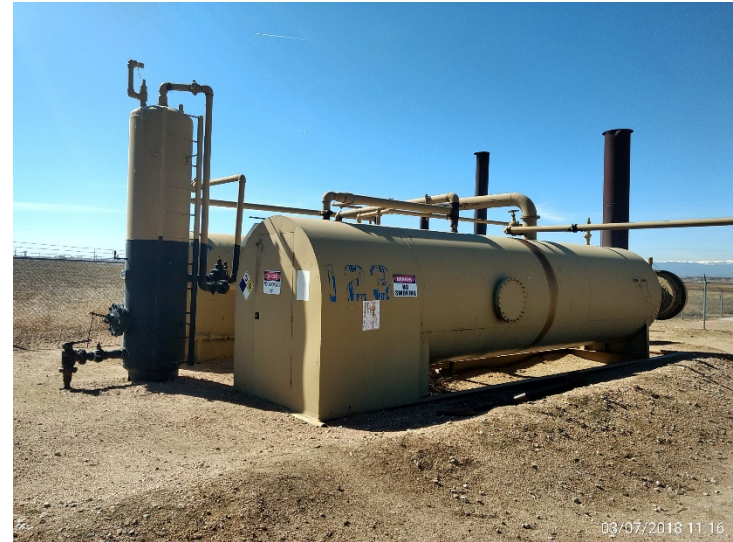
North Bulk Separators
