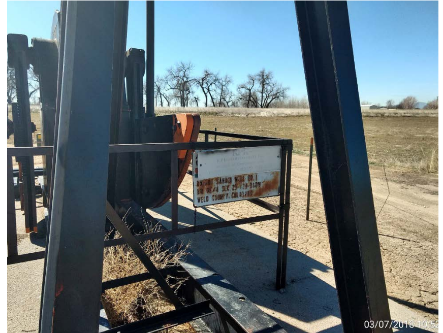
Wellhead Signage, Corrective action: Repair or Replace faded signage, per rule 210.b
