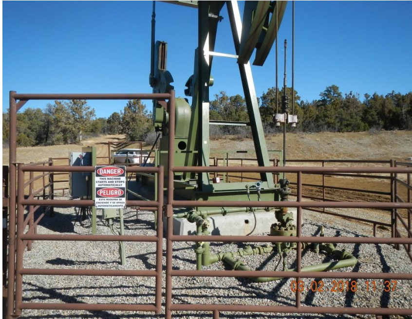
Royce State #36-2 pump jack and well head.
