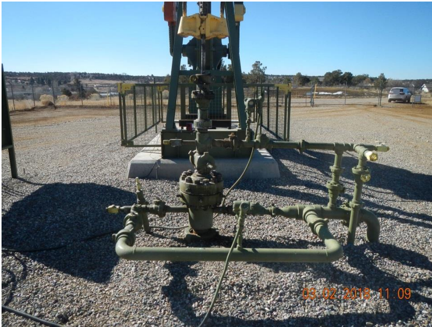
Well head is stained with white residue.
