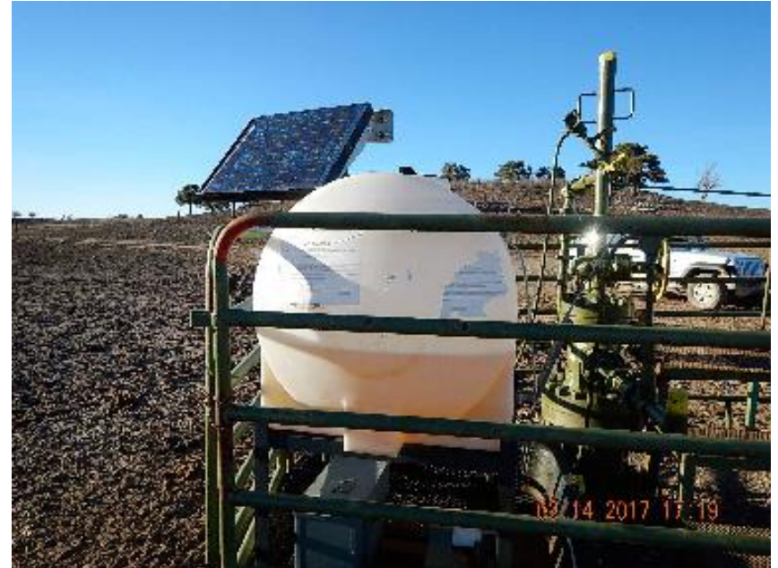
Photo 4: Glycol tank with no NFPA label previous inspection.
